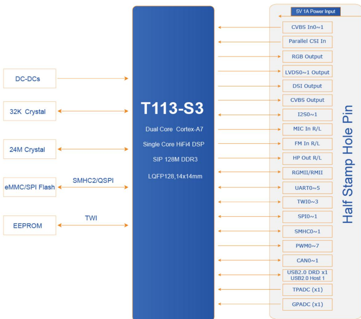
Figure 2-2 Core board block diagram
