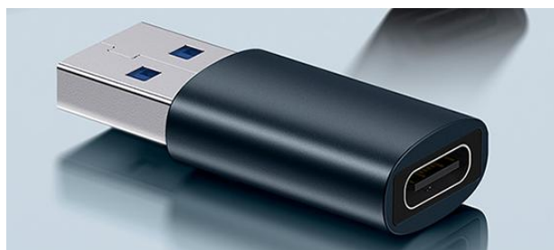
Figure 5-1. USB to Type-C Adapter Diagram
