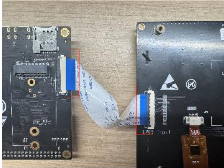
Figur 3-4. Connection between J6 and LVDS screen
