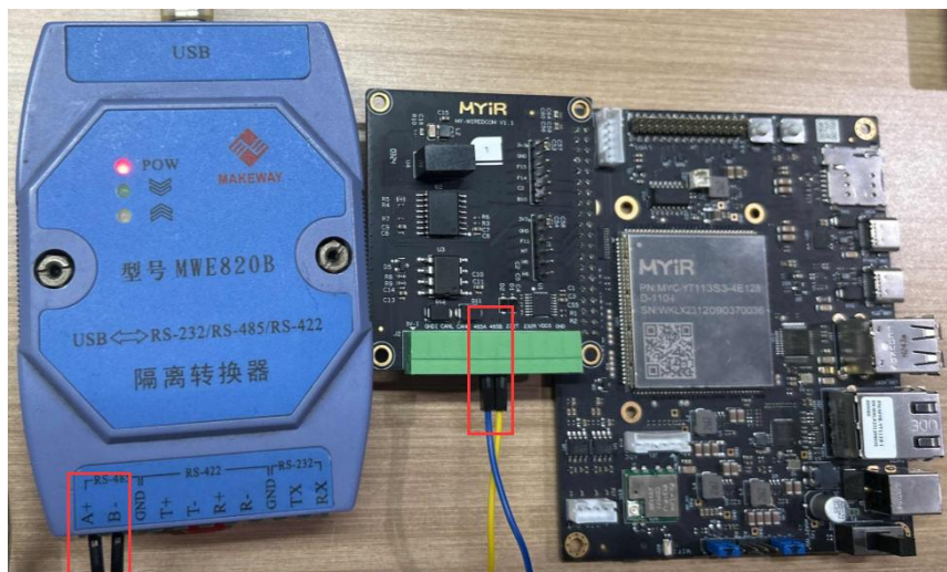
Figure 4-2. RS485 connection
